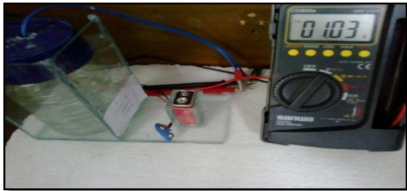
Figure 6: Stable output voltage of fuel cell kit
