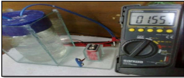
Figure 5: Fuel cell output voltage just after disconnecting battery supply
